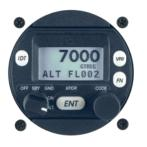
controller can be installed in a standard 21/4 inch instrument cutout, or where space is really tight it can fit a compact cut-out just 42mm high. Only a few centimetres are needed behind the panel to allow room for the connector and the static port interface. The transponder box itself is also only 45mm high, 62mm wide and 141mm long, and can be installed anywhere convenient in the airframe. A lightweight cable connects controller and transponder; it can be as long as you need.
