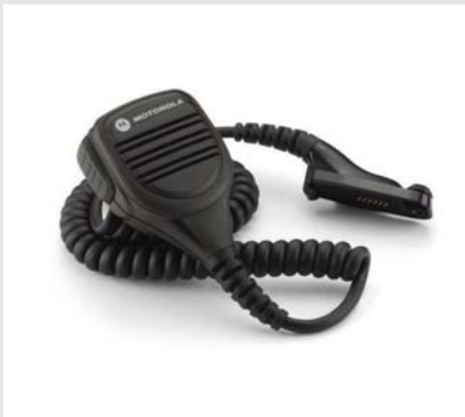
PMMN4080 IMPRES small windporting RSM with 3.5mm audio jack and emergency button, IP54.
