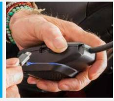
**DUALMIKE** can be recharged via the USB socket on the microphone or from the CB socket connected to the USB socket of the cable.
