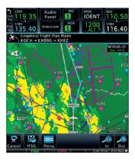
Graphical flight planning. Onscreen flight plan editing makes it easy to add waypoints or modify your route. And with handy "rubber band" feature, you can even stretch a flight plan leg to detour or amend your routing
