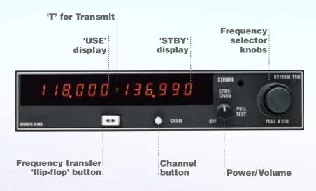
the transmitter and flashes the display if the mike is keyed for more than two minutes. (This prevents you from inadvertently jamming a frequency and making it unusable for other pilots.) There's also a 'Program Secure' mode that lets you lock a specific frequency into a specific channel number, so the program can't be changed from the panel.
